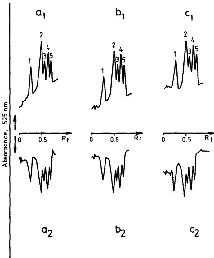
Fig. 9. Separation of quaternary ammonium compounds by two-directional linear OPMLC on three sorbent layers. Chromatographic conditions as in Fig. 7. ( $a_1$  and  $a_2$ ) Upper plate; ( $b_1$  and  $b_2$ ) second plate; ( $c_1$  and  $c_2$ ) lower plate. 1, TML; 2, choline; 3, carnitine; 4, trigonelline; 5, betaine.
