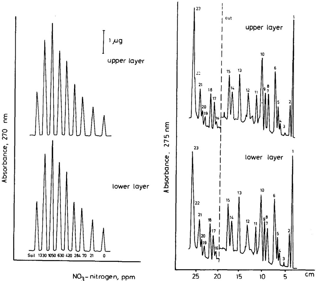
Fig. 10. Determination of trigonelline in tomato leaf extracts with different  $\text{NO}_3\text{-N}$  levels by OPMLC on two sorbent layers. Chromatographic conditions as in Fig. 7, except quantitative evaluation at 270 nm with Shimadzu CS-930 scanner.
